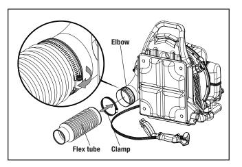
2. Install flex tube to tube with upper blower tube (with the throttle handle guide). Use the slightly smaller clamp with diameter of 59-82mm. Tighten the clamp fully.
