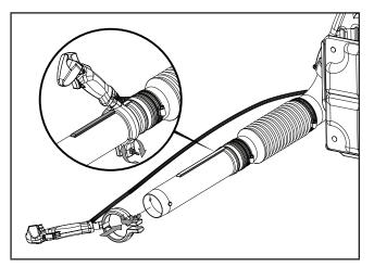
4. Assemble upper blower tube to middle blower tube by aligning the arrow of the peg of tube with the arrow of the locking groove of tube. Slide the peg into the locking groove and rotate clockwise to lock in place.
