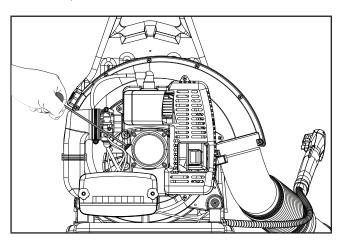
6. Move choke knob to the RUN position and pull recoil starter handle until engine starts. Do not pull more than 6 times.
