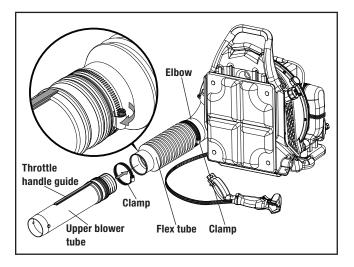
Loosen wing nut completely on throttle handle clamp. Align notches in throttle handle clamp with guide on the upper blower tube and slide on as shown. When the throttle handle is at the desired length, tighten the wing nut fully to secure.
