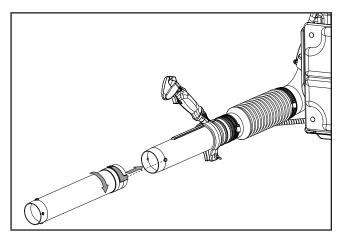
Assemble middle blower tube to lower blower tube by aligning the arrow of the peg of tube with the arrow of the locking groove of tube. Slide the peg into the locking groove and rotate clockwise to lock in place.
