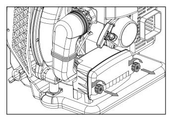
3. Inspect and replace or clean the air filter. To reassemble make sure the filter fits in the cavity and reinstall the filter as shown. Fasten the air filter cover by turning the fasteners clockwise.
