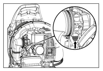
4. Engage the throttle trigger and safety lock while pushing the throttle lock inwards.
